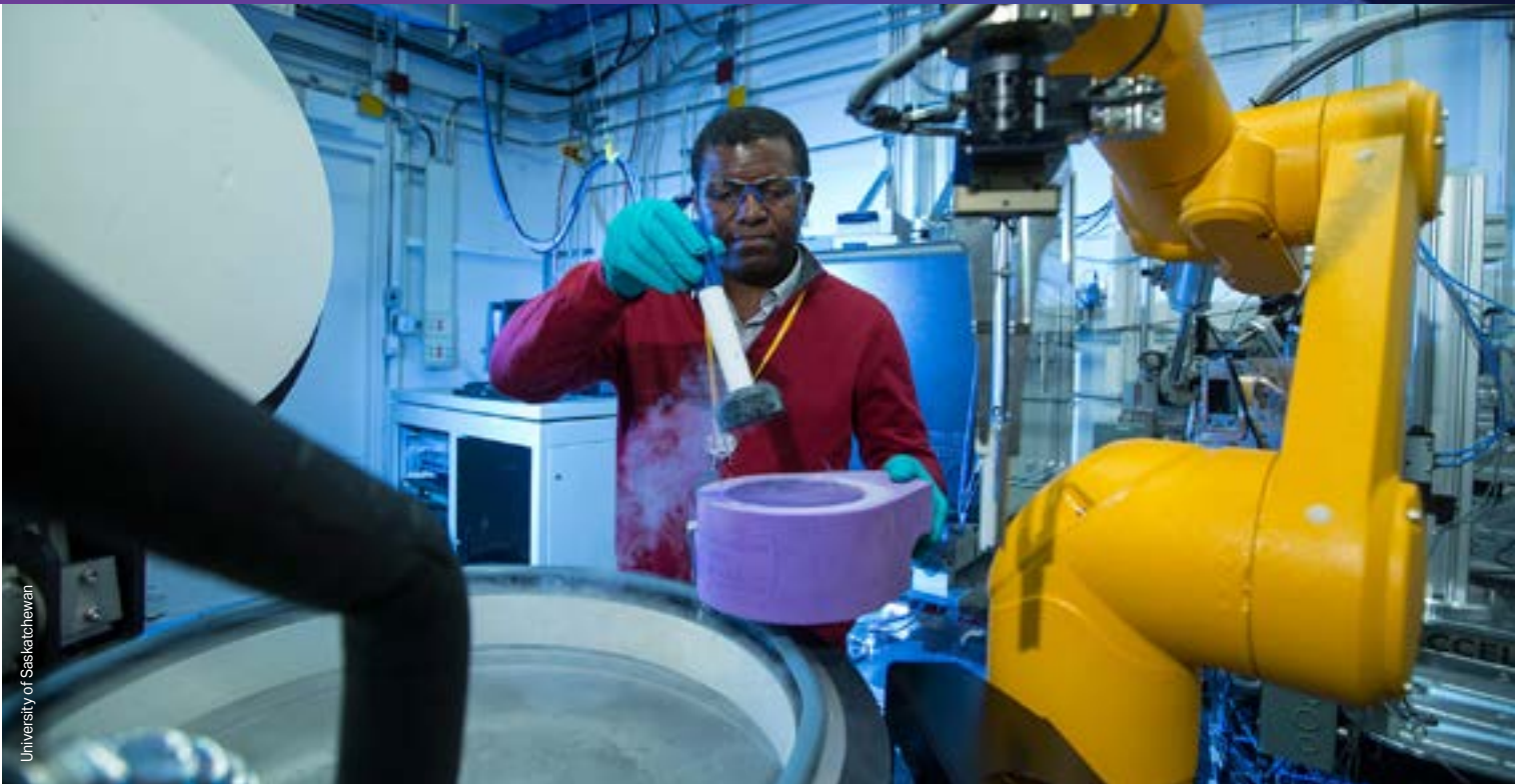
Michel Fodje, Senior Scientist at the Canadian Light Source synchrotron facility at the University of Saskatchewan in Saskatoon, Sask., loads samples into a robotic sample mounter on the structural biology beamline, which is used for drug development and to study diseases.
